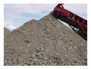
Locate plant for processing where you want the stockpiles to be located to save moving stockpiles later. As the pile reaches the height of the conveyor, the plant will need to be moved to the next stockpile location.
