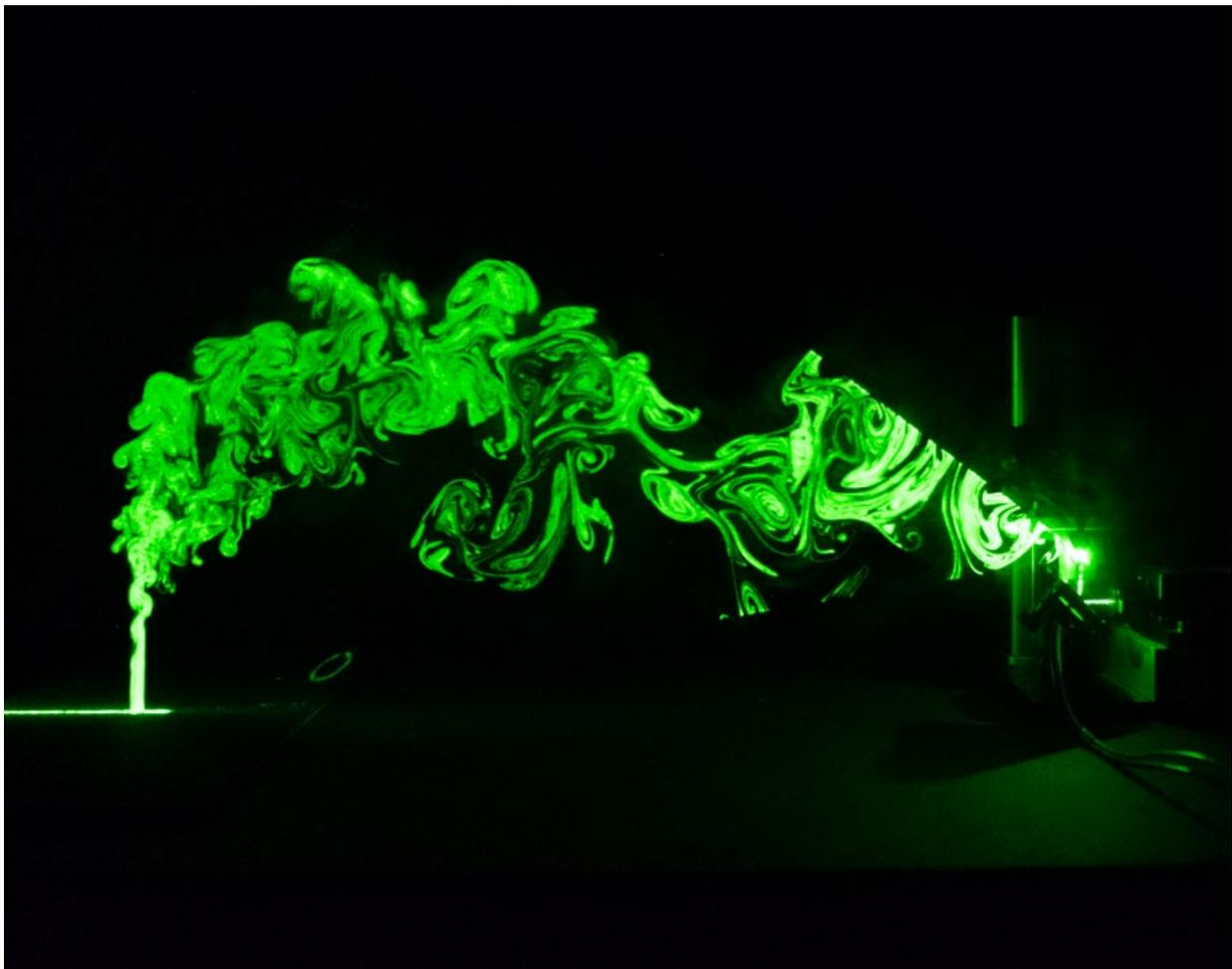
Demonstration of air flow through ceiling penetration at the mean ceiling-roof cavity pressure difference of 1.2 Pa using smoke and LED light.
