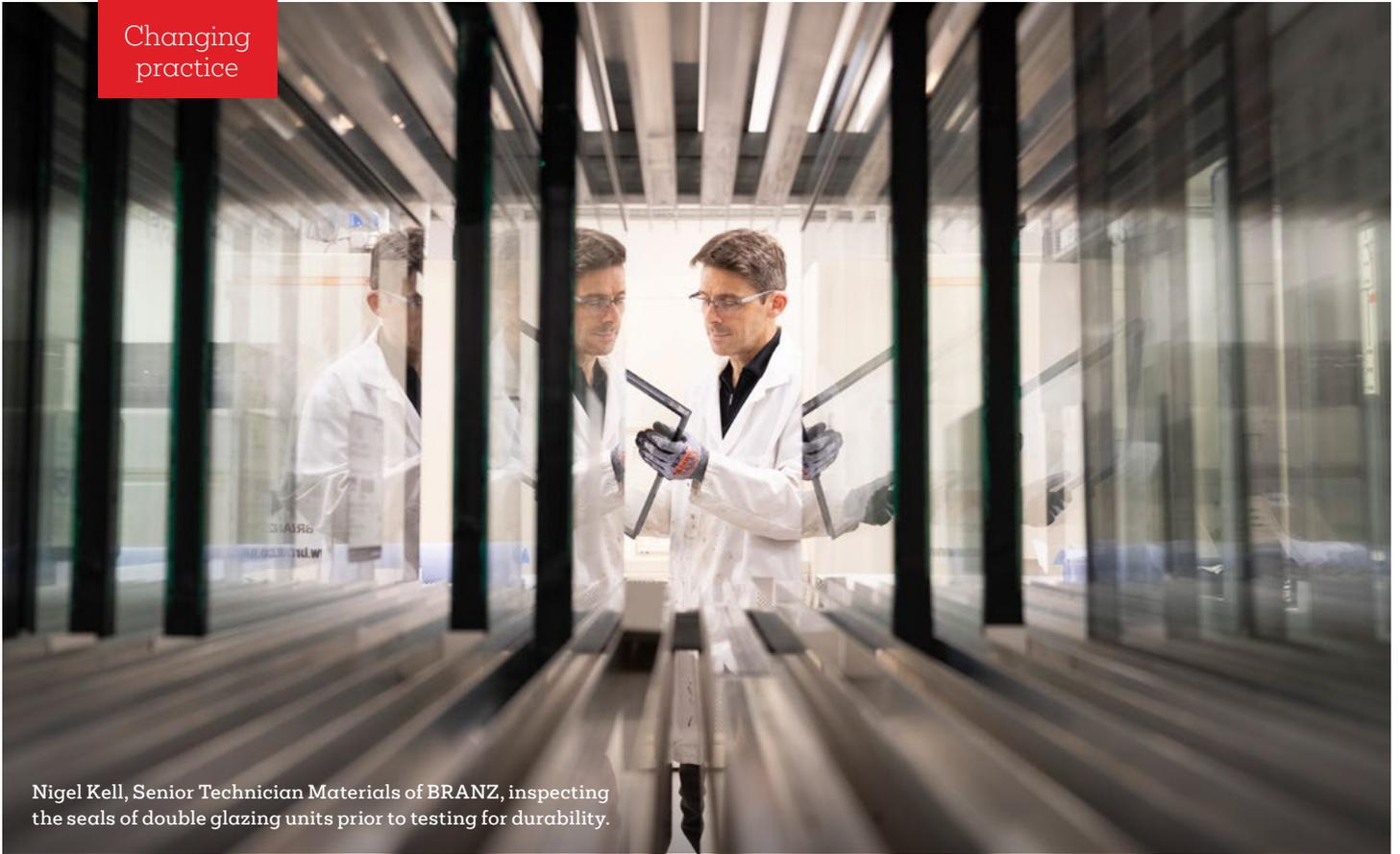
Nigel Kell, Senior Technician Materials of BRANZ, inspecting the seals of double glazing units prior to testing for durability.
